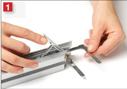
1 Lift FASTclamp lever and fully insert the 90° L-bracket. Lock clamp by pressing lever back down into the channel. Repeat for both clamps on this frame profile.
