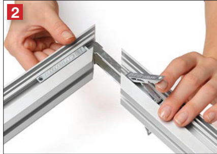
2 Insert the brackets of the first profile into the Fastclamp grooves of the second profile.
