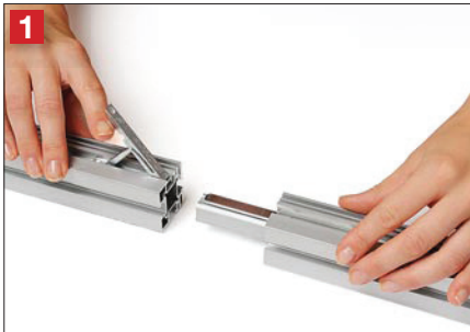
1 Lift the FASTclamp lever while inserting the profile stem. Make sure that the small metal bracket is in direct contact with the FASTclamp.
